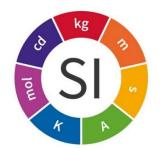
The SI Units (International System of Units) were globally agreed in 1960 and cover every type of measurement, the base units are shown in the diagram.
